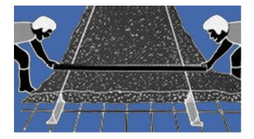
SHAPING OF CONCRETE - Manual Rule or Vibrator.
