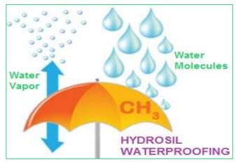
What makes this "umbrella" unique is its ability to breathe. Because siloxanes/silicones have a very open molecular structure, water vapor trapped in the substrate can easily slip through. Water molecules, however, are too large to enter.
